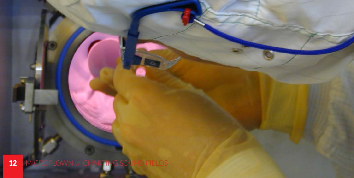
Production of Microflown sensor elements on silicon wafers
